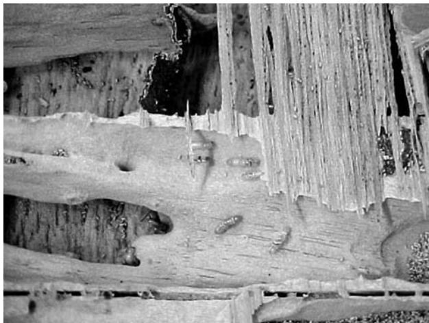
Figure 4.11. Insect attack on wood. Remnants of wooden cupboard door after attack by drywood termites ( Cryptotermes brevis ). Photo: Dr Neiva Barros, University of Caxias do Sul, Brazil.
