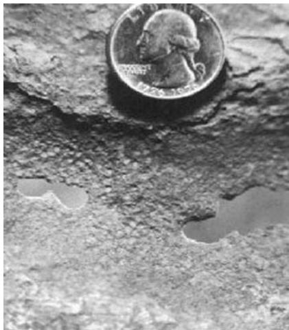
Figure 3.30. Steel pipe corroded through within 2 years of being placed in an anaerobic soil. Photo: Dr Christine Gaylarde.
