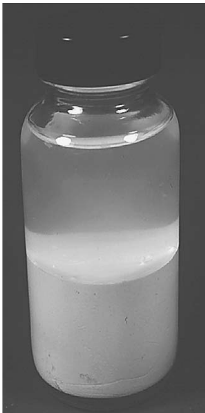
Figure 3.22. ‘Split’ emulsion paint. Photo: Dr K. J. Seal.
